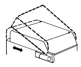
A. To open battery compartment, slide lid toward handle and lift up. (Battery compartment is located on bottom of projector.)
