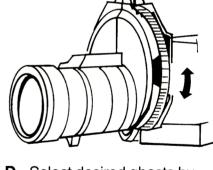
D. Select desired ghosts by rotating cartridge in projection slot. (To have sound without picture, rotate cartridge until light is blocked.)
