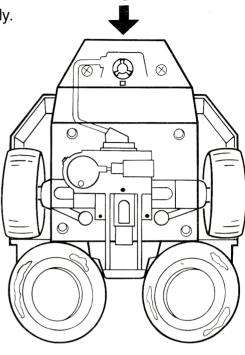
3. Assemble containment lid by inserting one peg at a time and snapping it into place.
