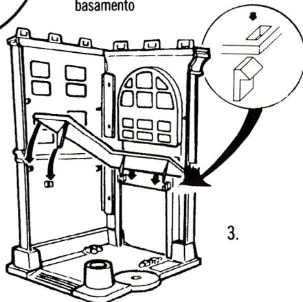
3. Snap second floor platform into place by sliding slots into floor brackets.
